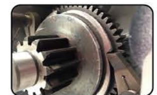
Double-lock brake system
